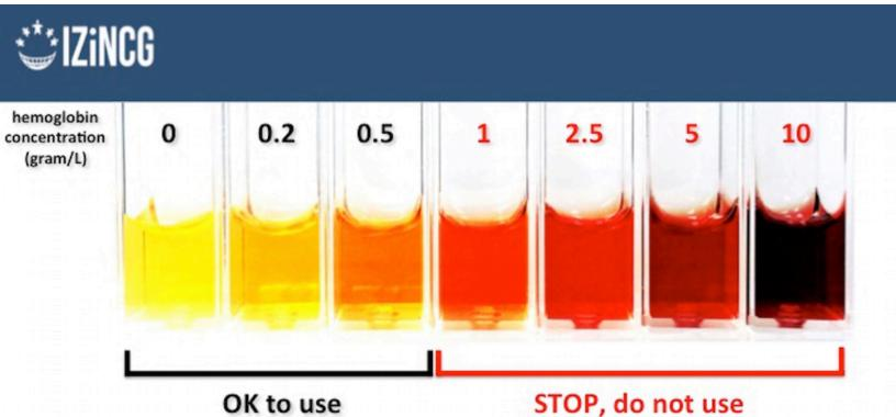
Hemolysis can contaminate plasma or serum samples with zinc.
